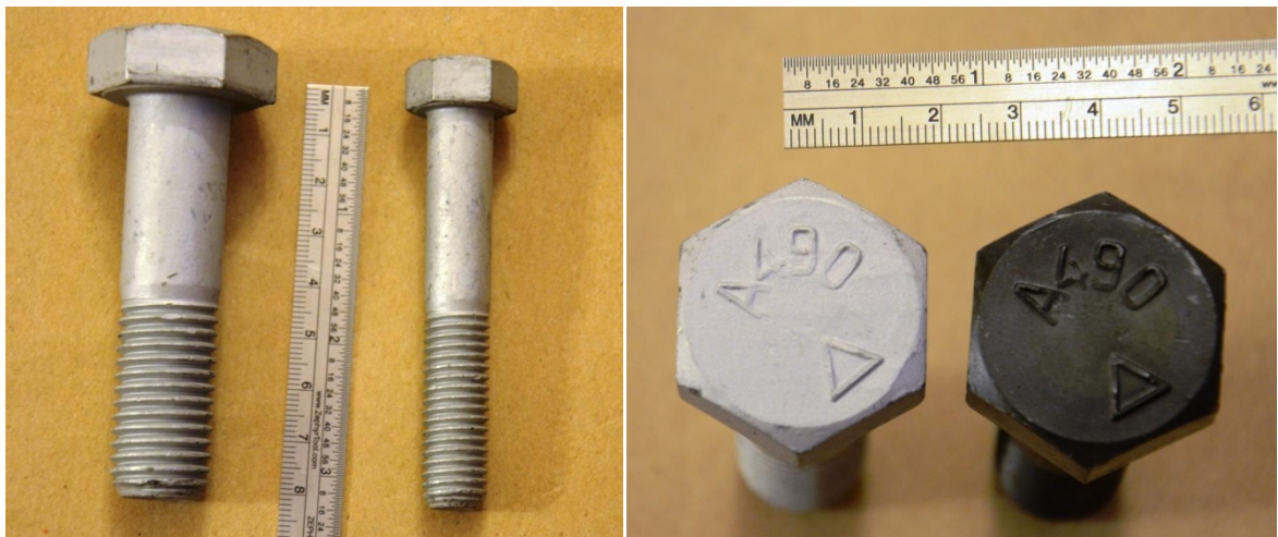
Figure 1 – Coated specimen bolts 3/4-10 x 3 and 1/2-13 x 3 (left), and coated and uncoated 3/4-10 x 3 specimen bolts (right)
