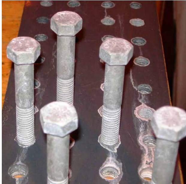
Figure 15 –1/2 inch bolts after 1000 h of salt spray exposure
