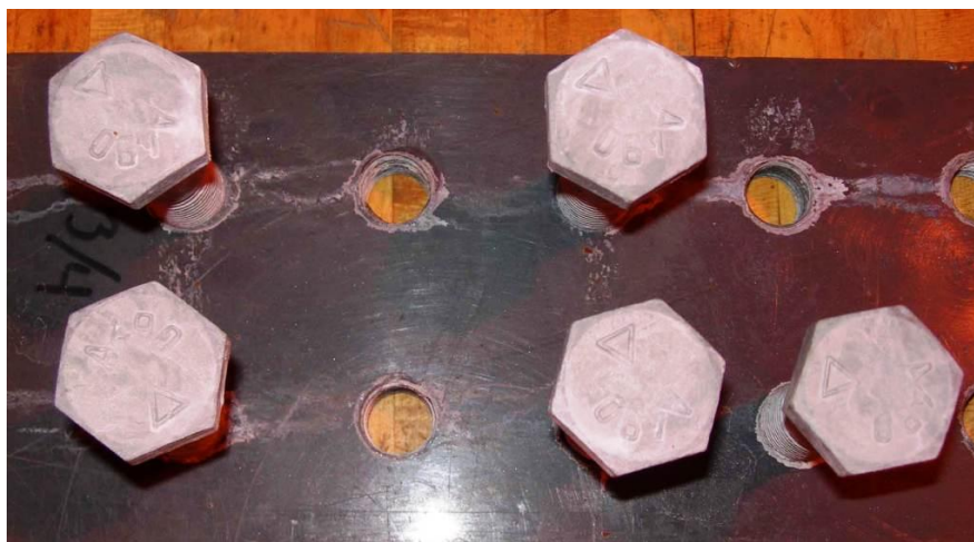
Figure 14 –3/4 inch bolts after 1000 h of salt spray exposure
